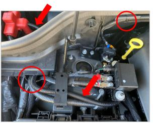
Route power cable from circuit breaker to factory battery/jump start point
