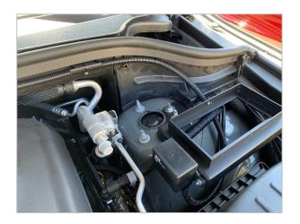
Bracket mounts to driver side strut tower utilizing two factory mounting locations.
