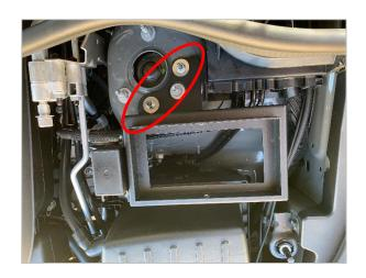
Mount panel utilizing two M6 nuts on factory studs on strut tower
