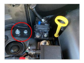
Mount circuit breaker using M8 and M6 nuts at factory location studs on strut tower
