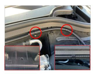
Route power cable from circuit breaker to Patrol Power panel as shown using cable ties and cable clamps. Loom, secure & protect all wiring.
