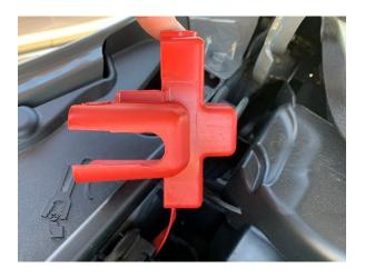
Trim cover for factory jump start point as shown for power cable clearance
